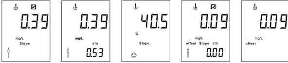
Dip the electrode into the test solution, the stabilized icon will be displayed at the top of the screen once the data stabilized. Press "ENT" to confirm.
