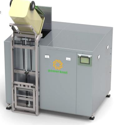
The LFC-1000 is a fully enclosed automatic biodigester that safely disposes of 1000–18000 kg (2200–4000 lbs) of waste food each 24 hours with no noise or odor. Once installed, you can use the bin lift to add waste at any time without needing to empty byproducts. The LFC discharges only decomposed food as grey water that is environmentally safe.
